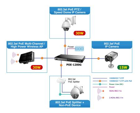
With data and Power over Ethernet from one unit, the POE-1200G can reduce power cable deployment and eliminate the need for dedicated electrical outlets on the wall, ceiling or any unreachable place.
