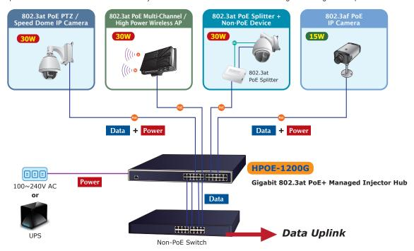
With data and Power over Ethernet from one unit, the HPOE-1200G can reduce power cable deployment and eliminate the need for dedicated electrical outlets on the wall, ceiling or any unreachable place.
