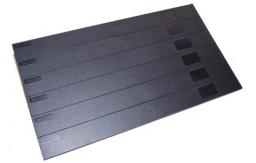
Fitting 19" blanking or EaziBlank panels (and deploying rack air anti-recirculation kits) helps to avoid air mixing and recirculation within the rack space which in turn helps to maximise the cooling infrastructure effectiveness by delivering cool air to the equipment and not allowing it to bypass through empty U spaces.
